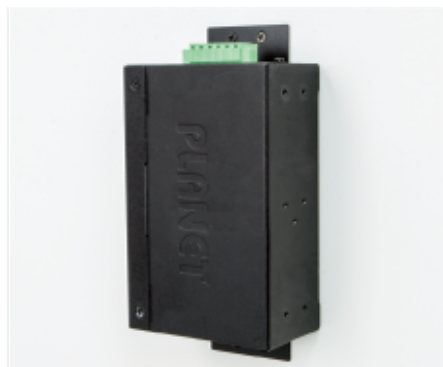
Side Wall Mounting (Space saving)
