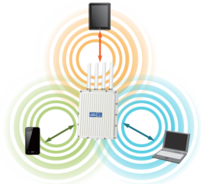
MU-MIMO Serving multiple users simultaneously
